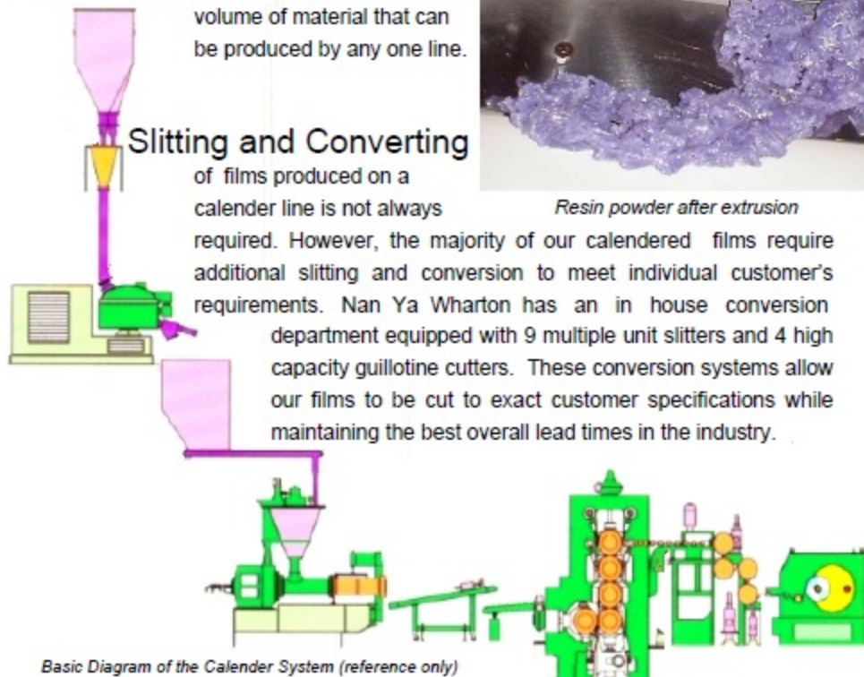
Basic Diagram of the Calender System (reference only)
