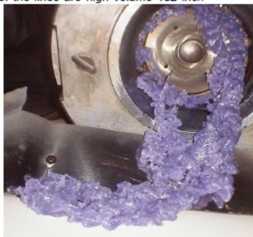
Resin powder after extrusion
